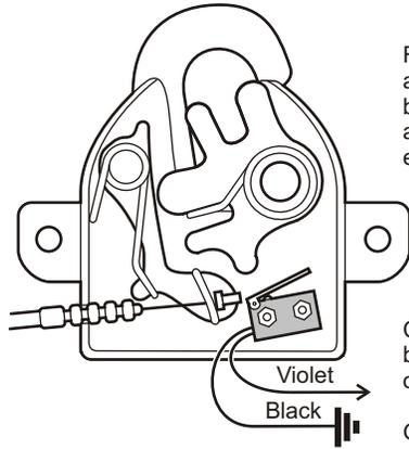
Remove bonnet lock assembly and fix bonnet switch using attached screws to existing holes
